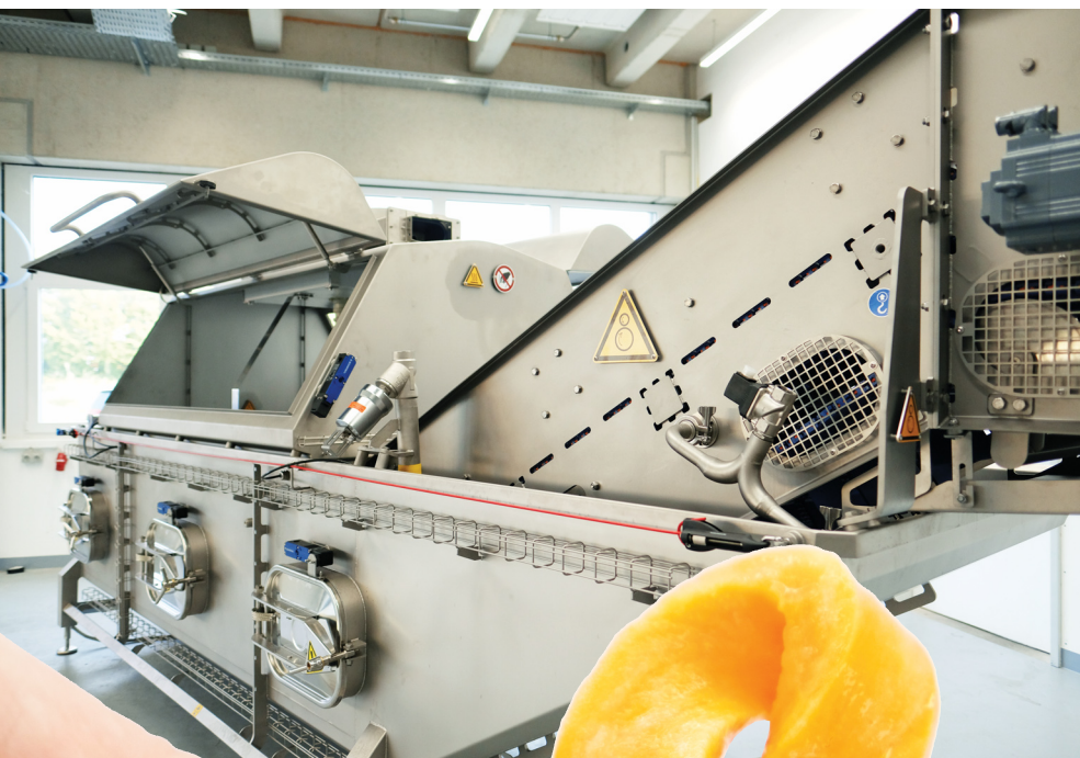
New Elea PEF Advantage B 1000-850 system processing up to 100 t/h
